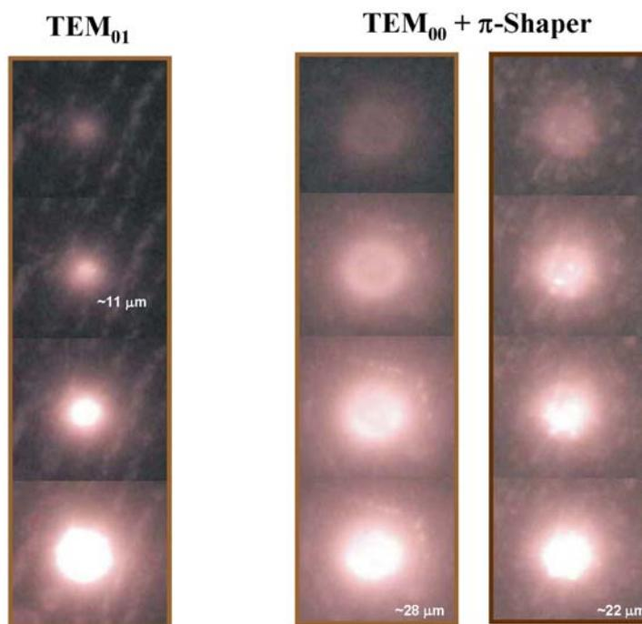
Evidently, applying the **F- $\pi$ Shaper 9\_1064** lets it possible to realize the **Flat Top Laser Heating (FT-LH)** and provide most stable conditions for experimental investigations of physical and chemical properties of materials.
