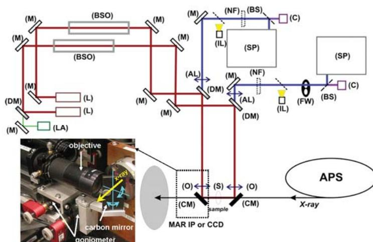
The initial Gaussian laser beam is converted, by means of the beam shaping optics **BSO** on the base of the **F- $\pi$ Shaper 9\_1064**, to the beam which intensity distribution is optimized to create the flattop profile on the sample **S**.
